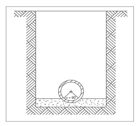
Between the trench bottom and the pipe a bedding angle of at least 90° must be realized with materials that can be compacted well.
