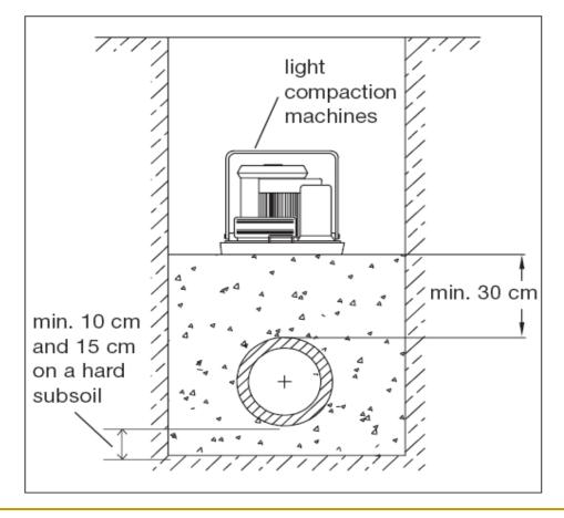
The selection of the compacting device, the number of passes and the thickness of the layer to be compacted should match the backfill material.
